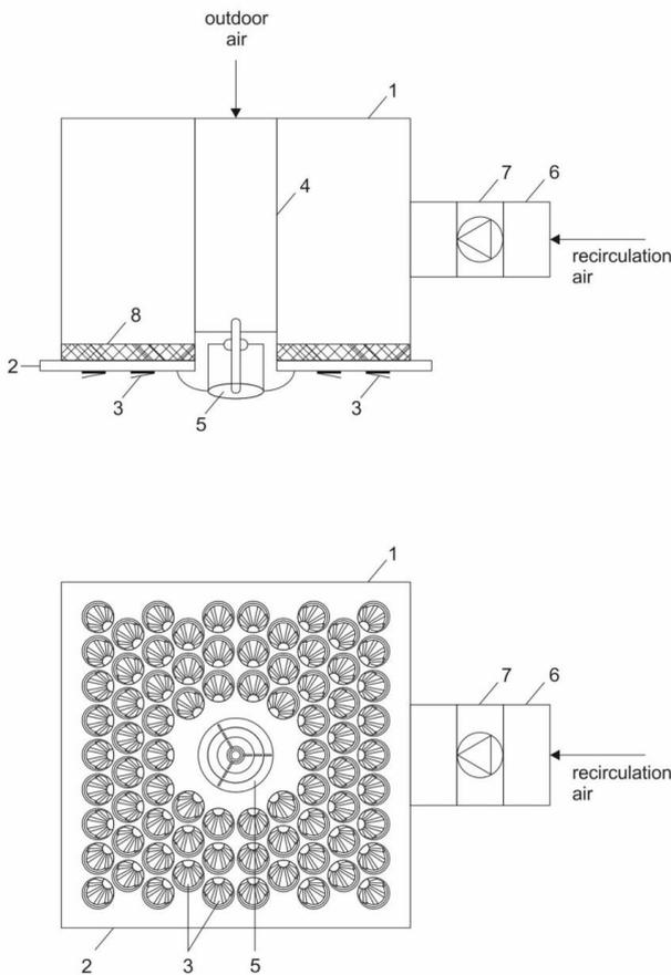
Figure 2. Schematic view of local recirculation diffuser.
