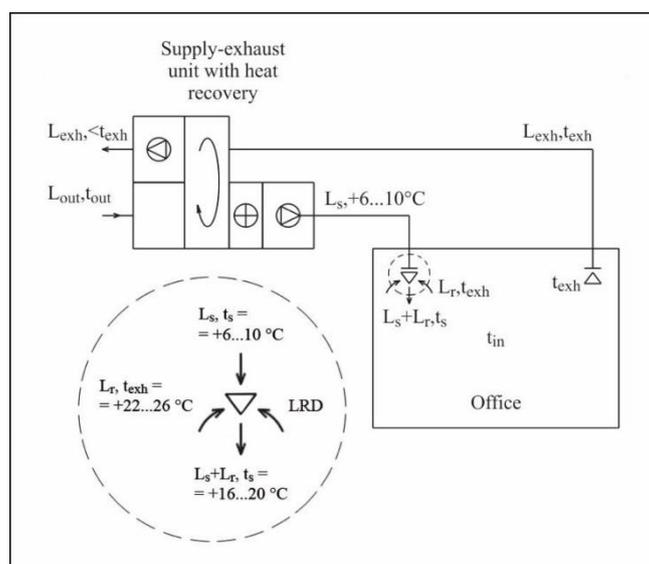
Figure 1. Schematic view of ventilation system with local recirculation diffusers.
