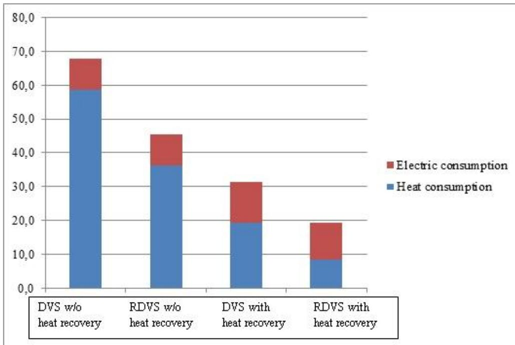
**Figure 3.** Specific annual energy consumption of ventilation systems, kW·h/m<sup>2</sup>.
